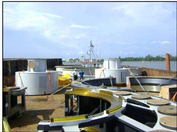
Surveyor inspecting the lashing and securing arrangements.
