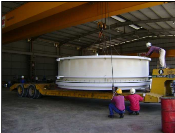
Loading of Dilatation piece on trailer.
