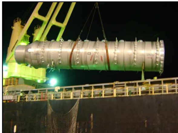
Deodorizer tank being loaded on MV.
